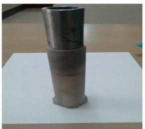
Fig-2.Composite shaft after machining
