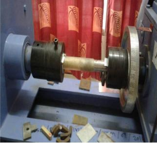
Fig-3.Experimental set up for torque testing
