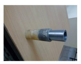
Fig-1.Composite shaft before machining
